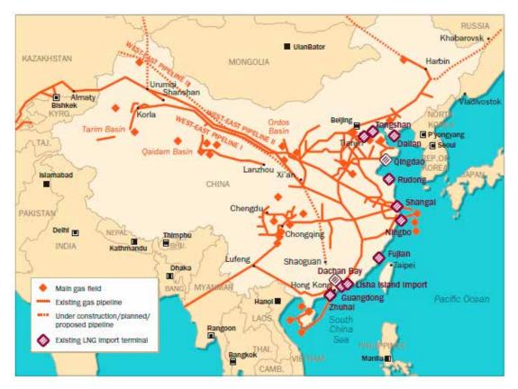
Source: China's gas supply infrastructure. Forecast: China Coal-to-Gas Project. Platts (January 2014). <u>http://www.platts.com/news-feature/2014/naturalgas/china-coal-to-gas-projects/index</u>
